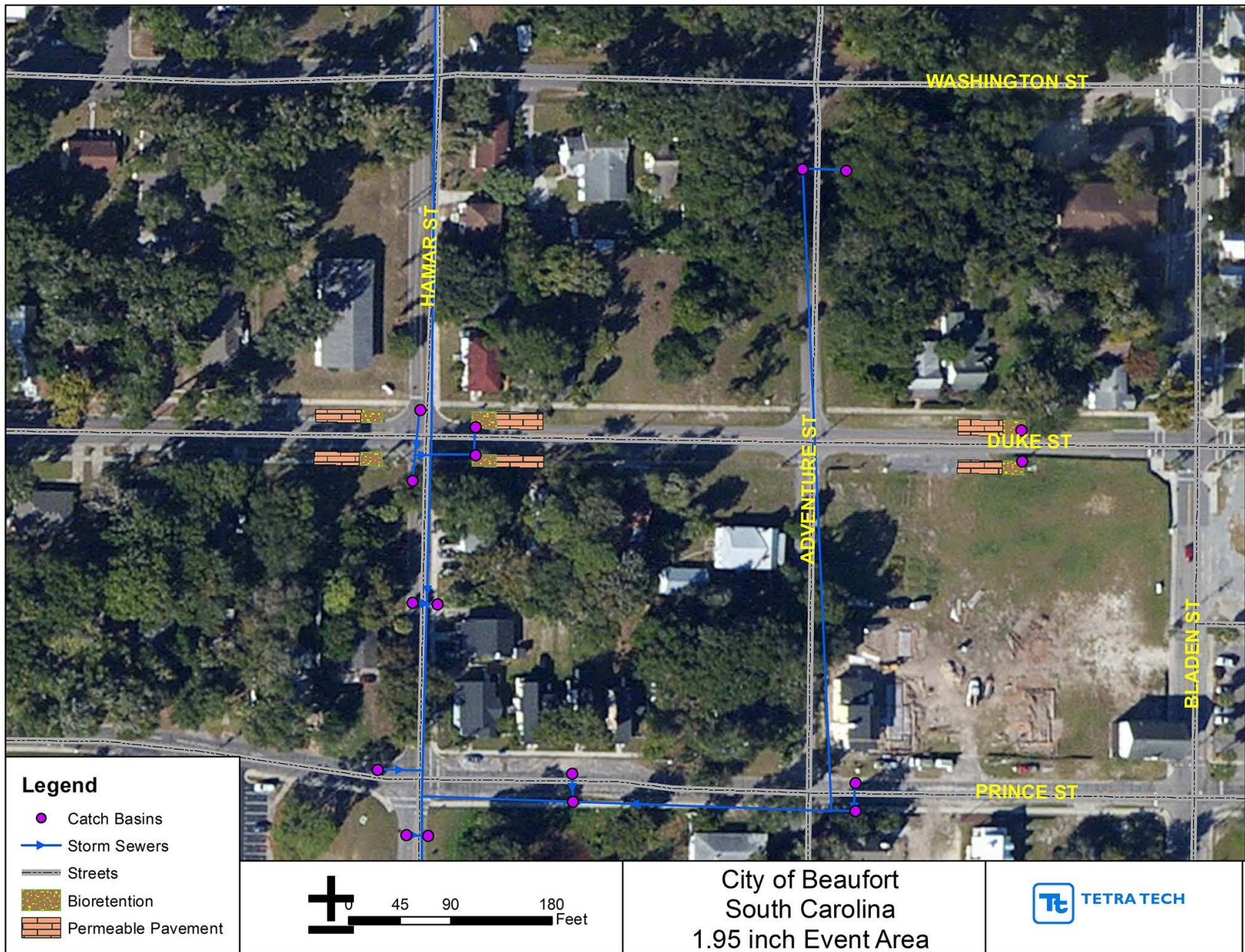
Figure 5-2. Recommended green infrastructure practice area on Duke Street to treat the 1.95 inch event.
