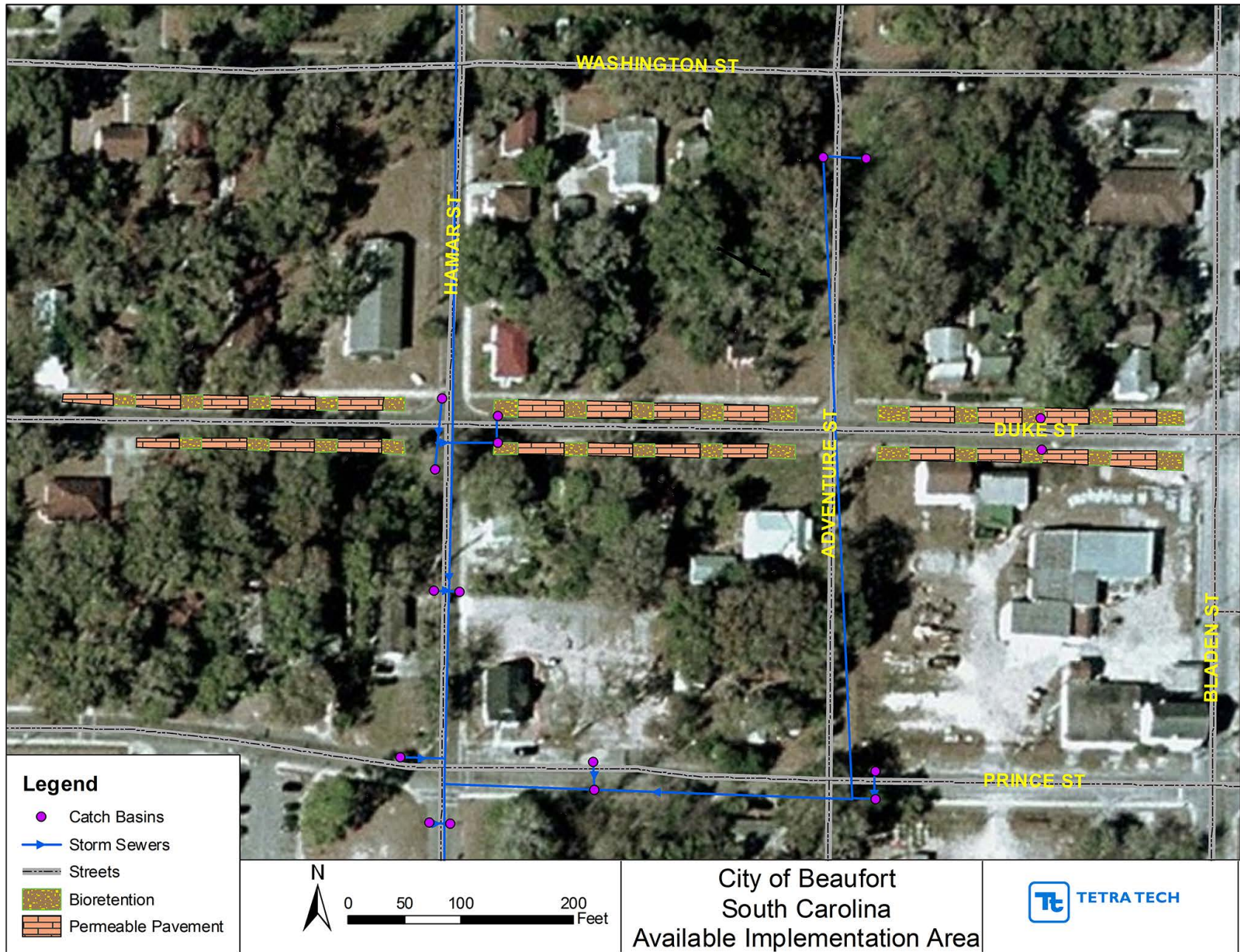
Figure 5-1. Available green infrastructure practice area on Duke Street.
