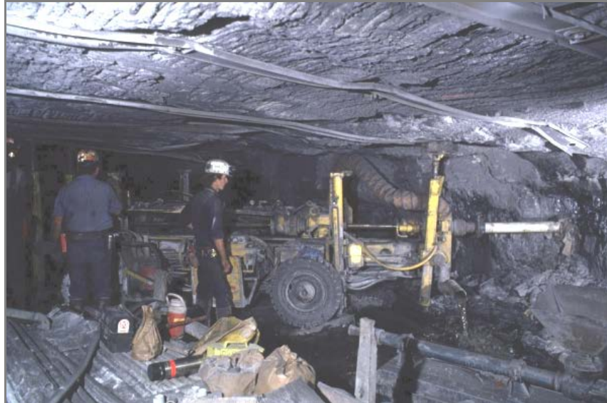
Exhibit 10: Longhole drilling from within a mine entry [JWR, 2008]
