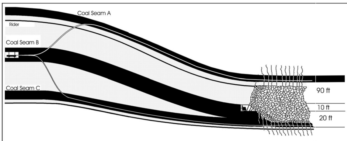
Exhibit 13: Superjacent boreholes reduce in-situ gas content and drain gob gas [Brunner et al., 2005]
