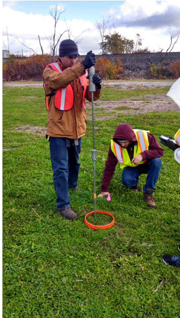
Figure 5. The field crew performs a penetration test using a single mass penetrometer.
