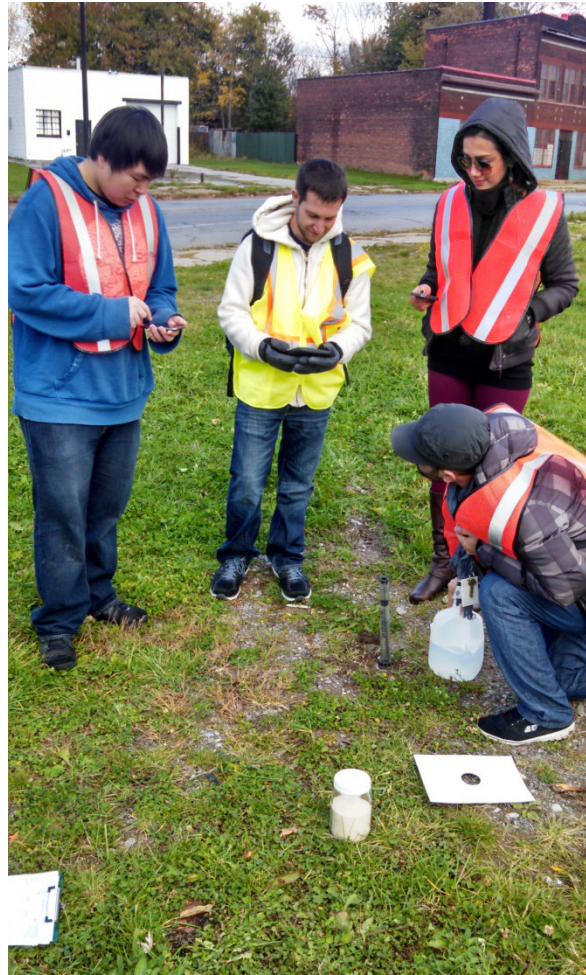
Figure 11. The field crew performs an infiltration test using a tension infiltrometer.
