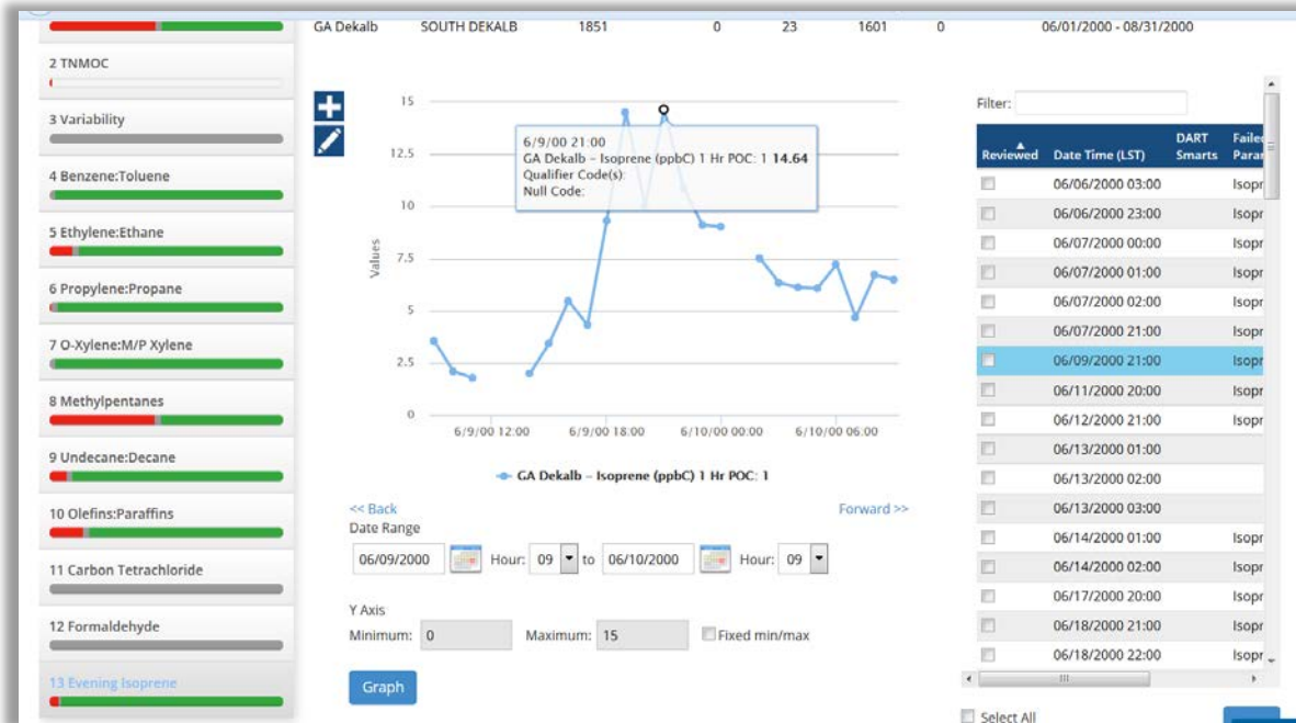
Figure 13. Example of unusual high nighttime isoprene concentrations. Typically, isoprene concentrations are highest when solar radiation and temperature are high. Because solar radiation is zero at night, these high concentrations may need further investigation.
