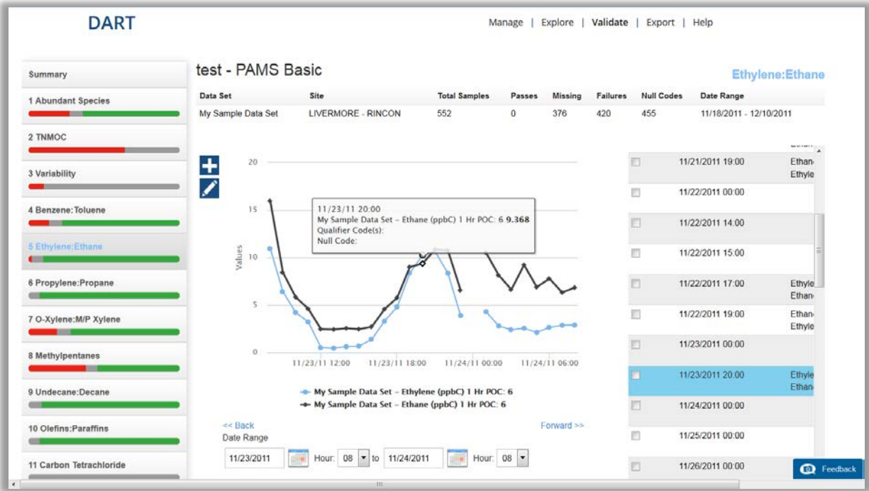
Figure 7. An ethylene:ethane ratio check. In this example, the ethylene concentration is greater than ethane concentrations. However, the concentrations are very close, possibly within the precision of the instrument, and at user discretion the data may be deemed valid.
