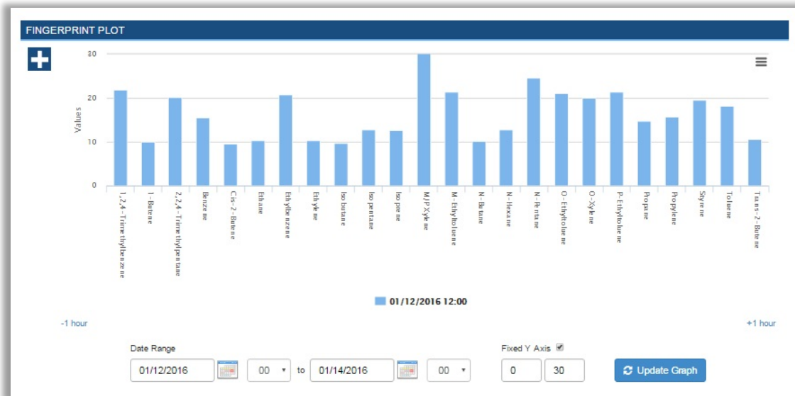
Figure 19. Precision check example showing that this fingerprint is quite different from a typical one. Higher concentrations are observed with all species present well above detection. This sample should be invalid and flagged as AX (precision check).
