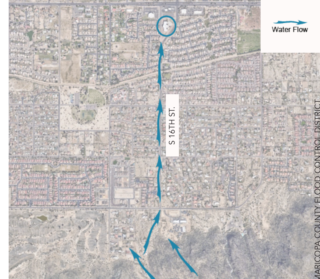
Heavy seasonal monsoon rains flows directly from South Mountain, north on 16th street, straight toward the schoolyard.
