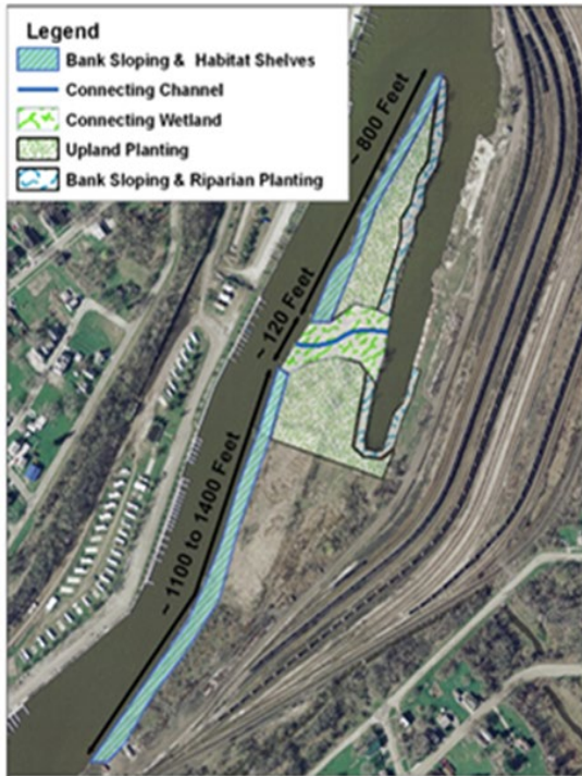
Figure 8. 5 ½ Slip Habitat Shelf & Upland Remedial Work
