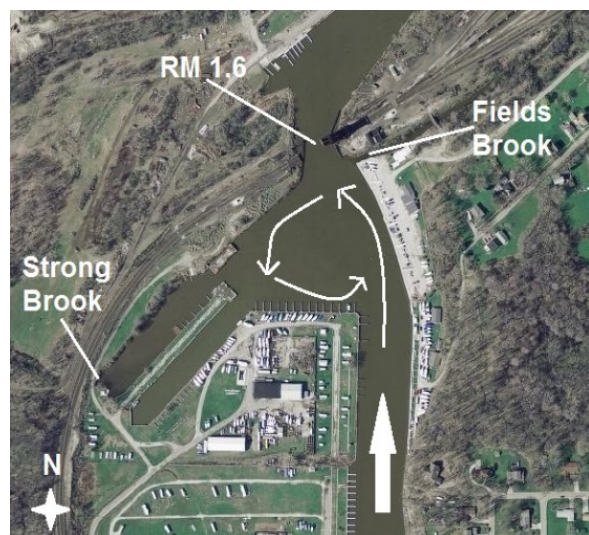
Figure 7. Cycling of river flow in turning basin
