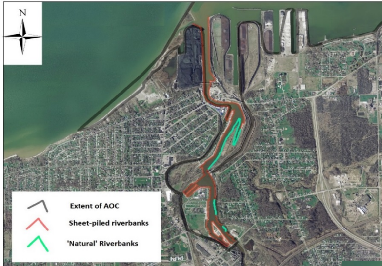
Figure 1. Sheet-piled and natural riverbanks in the Ashtabula AOC
