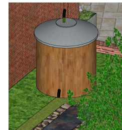
Figure 16 – Small above ground cistern in the outdoor lab in Area 3.
