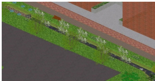
Figure 12 – Isometric view of the Bioswale between EMCS building and Reserved Parking lot in Area 4.
