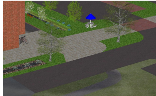
Figure 18 – Permeable sidewalk, parking pavers, and porous asphalt next to the EMCS and adjacent to the student parking lot and bioswale in Area 1 and Area 2.
