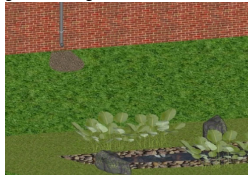
Figure 11 – Downspout Disconnect to Rain Garden between building and parking lot in Area 2.
