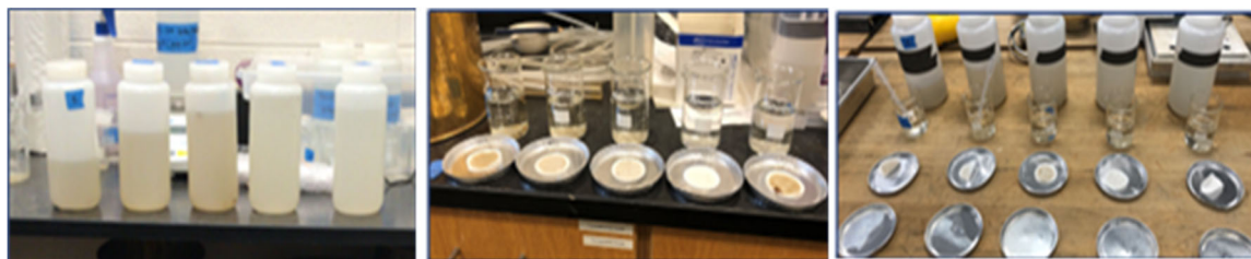
Figure 7 – (Samples from left to right) 1. Initial water samples collected on site; 2. Test of suspended solids; 3. Final result of all samples showing dissolved solids
