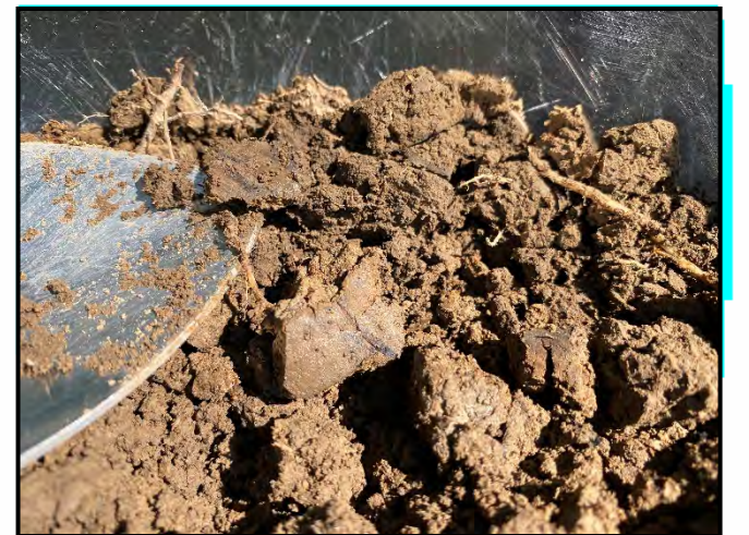
Photo 103: Closeup of KD275SS-(1 and 2) showing dark streaks in soil.
