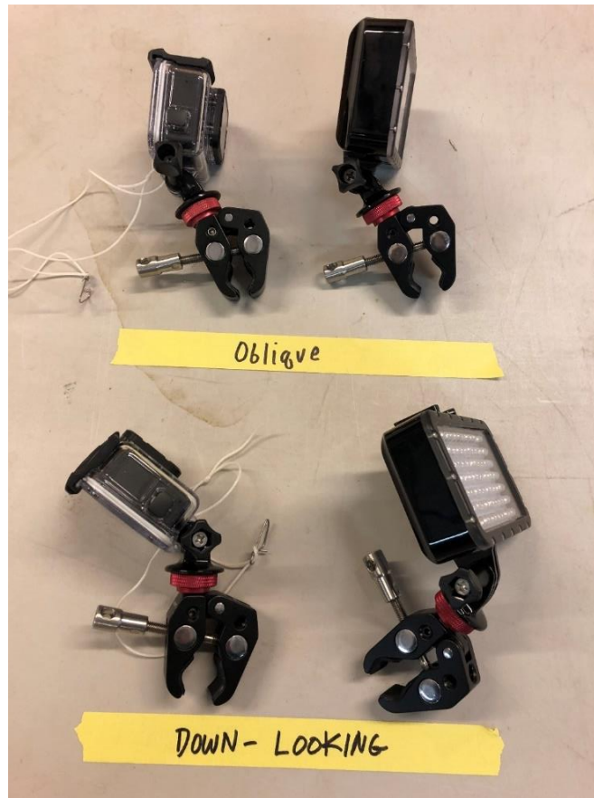
Figure 12.3. Approximate aiming angle of camera and lights for the oblique (B) and down-looking (A) cameras. Note the orientation of the tripod adapter (the fitting between the red locking thumbscrew and the camera or light) which is facing backward relative to the camera lens.
