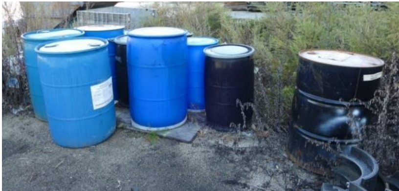
Chemical drums not properly labeled and no secondary containment.
