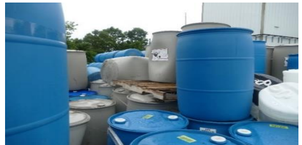
Chemical drums improperly stacked and some drums under duress.
