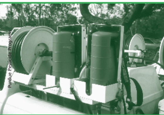
Lock backpack sprayers securely onto the transport vehicle.
