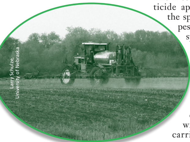
A hydraulic sprayer with a spray boom.
