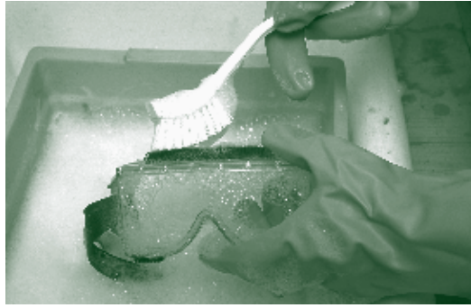
Clean goggles, face shields, and respirator bodies and facepieces in detergent and hot water.
