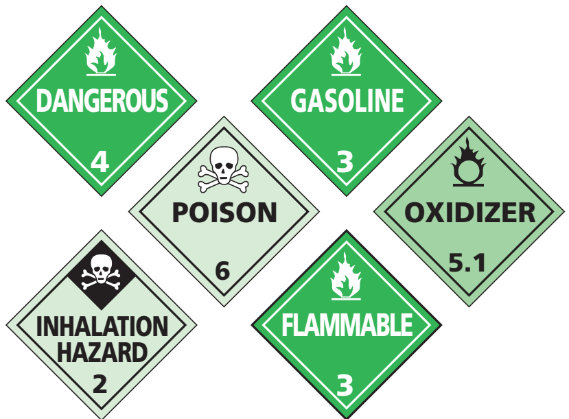
Examples of placards placed on vehicles that transport certain types of hazardous materials.
