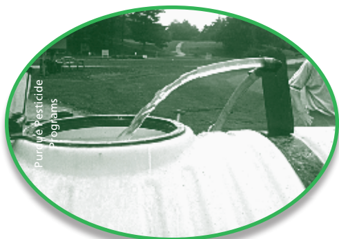
Leave a distinct air gap between the hose and the surface of the pesticide mixture to prevent back-siphoning.
