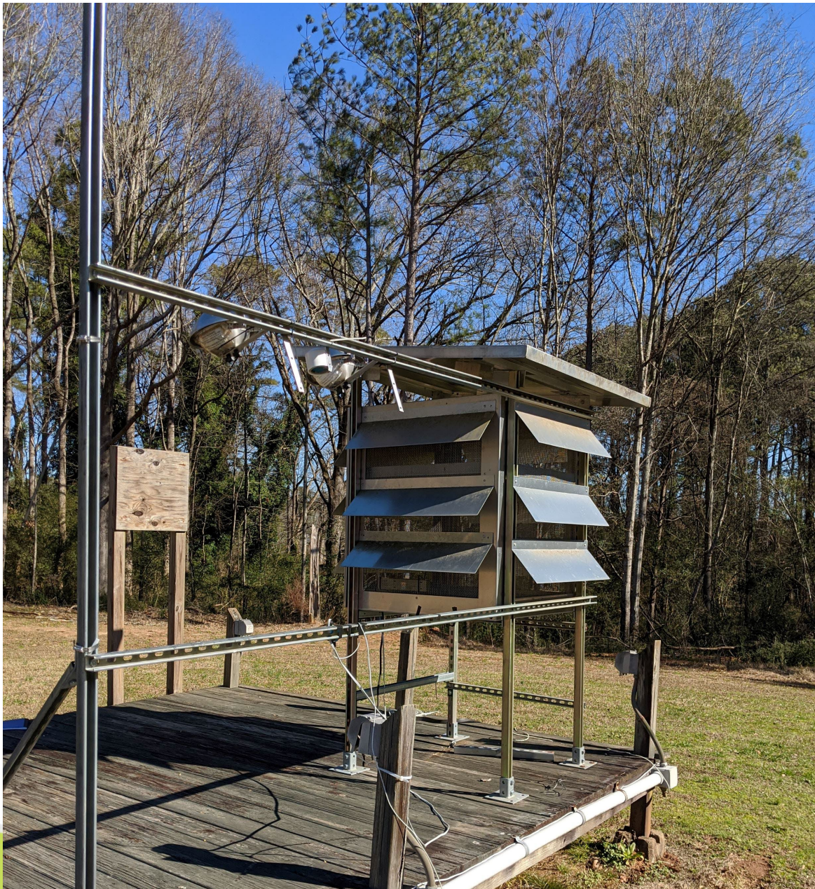
Collocation Shelter installed in Atlanta, Georgia
