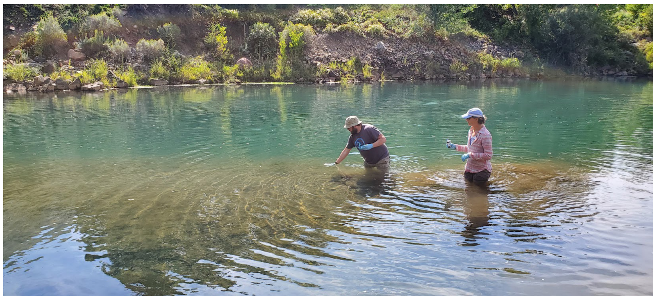
EPA scientists Richard Mitchell and Shera Reems collect water samples from the Animas River in Colorado. The samples will be analyzed for PFAS and other contaminants as part of a collaborative project between EPA, four states, and three Tribes to identify contaminants in the San Juan watershed.
