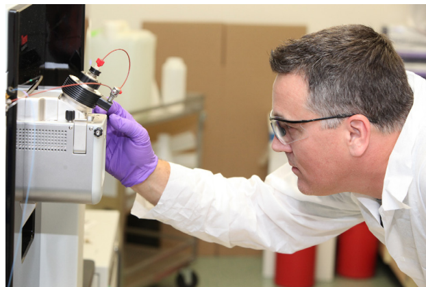
Mark Strynar from EPA's Office of Research and Development monitors a high-resolution mass spectrometer while conducting non-targeted screening for emerging PFAS.
