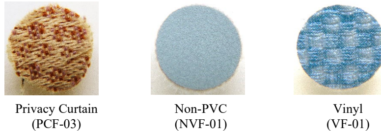
Figure 1: Examples of carrier materials cut into 1 cm discs; materials 2.a.i, 2.a.ii, and 2.a.iii (from left to right)
