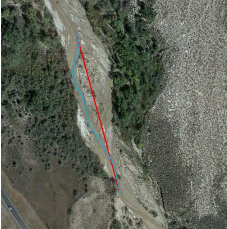
Figure 19. Sinuosity measurements in a multi-threaded system. The stream length (dashed blue line) is measured in the dominant (i.e., lowest elevation) channel. Valley length is represented by the solid red line.
