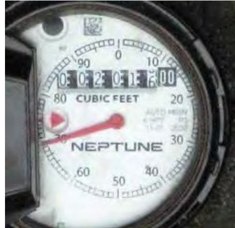
This meter reads 201,670 cubic feet
