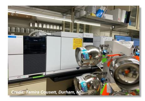
GC: Agilent 7890A MS: Agilent 5977B/Turbopump Source: Inert Plus Extractor Preconcentrator: Refurbished Entech 7200
