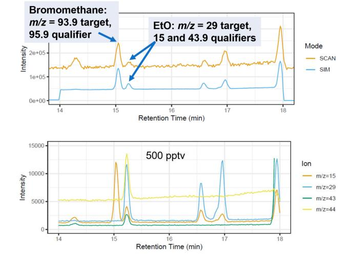
Note: Results from 7890A GC–5977B MSD using VF-624ms column.
