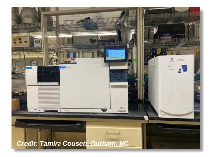
GC: Agilent 8890 MS: Agilent 5977C/Diffusion Pump Source: Inert Plus Extractor Preconcentrator: Entech 7200A
