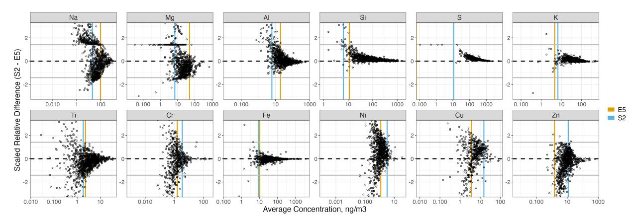
The vertical lines are MDLs colored by instrument models; The gray horizontal lines are  $\pm\sqrt{2}$
