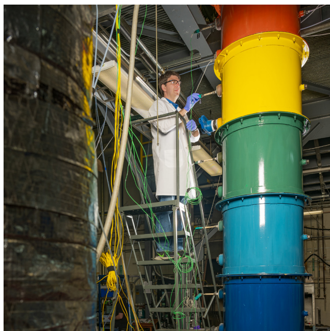
EPA researcher Erin Shields testing at the "Rainbow furnace," the EPA's innovative, pilot-scale tunnel incinerator, designed to test the effectiveness of PFAS destruction by incineration.
